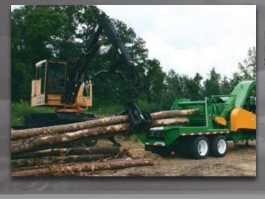
Options: All Husky models are available for trucks, stationary electric, rubber tire self propelled, and trailer-mounts. Husky provides the hydraulic power and control valves, oil lines and couplings for any major manufacturer's delimbers or slashers. We will custom mount on your choice of trailer.
