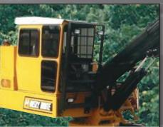
Improved access cab door, 38" x 60" floor dimensions, heater/ defroster, engine gauges, hydraulic system, warning lights, insulation, tinted glass, windshield wiper/washer, dome light, horn, fire extinguisher, cigarette lighter and ashtray.
