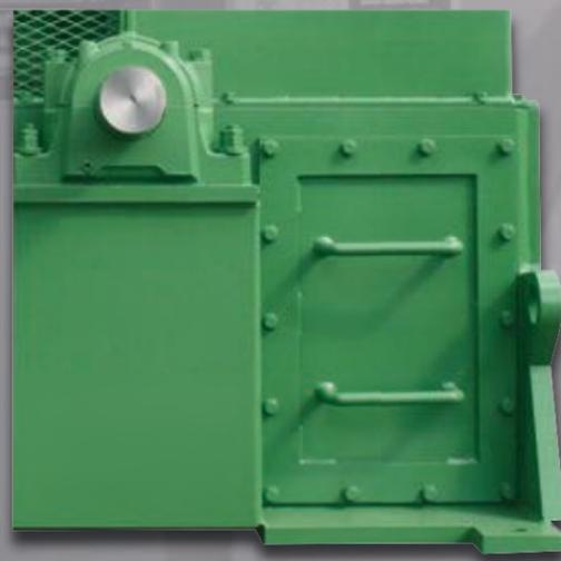
Optional Heavy-Duty Package: Includes chipper base with 1-3/4" (45mm) or 2" (51mm) thick bolt-in replaceable back. (Thickness depends on chipper model)
