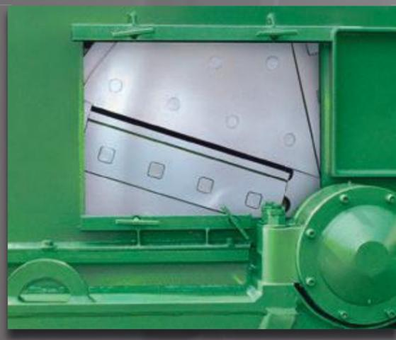
Knives are easily changed through large access door in front section. Easily removed clamp type knives are standard.
