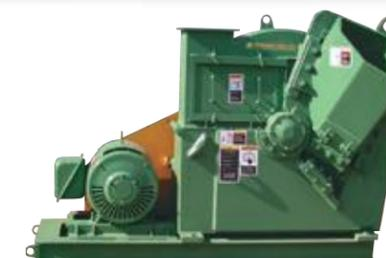
Drop Feed w/ Common base, motor and guards.
