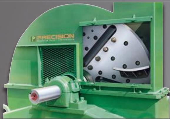
Rear section opening is opposite front opening with easy access for knife changing. Fan blades are easily inspected or changed.
