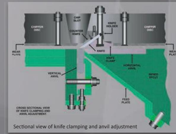
Sectional view of knife clamping and anvil adjustment
