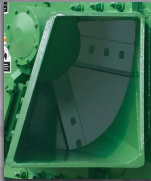
Larger infeed spout allows for increased capacity for both slabs and round wood.
