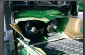
250 HP Diesel Engine. Multiple Different Hammer Options for Grinding Versatility. Tub Tilts 90 Degrees for Easy Access to Hammermill, Screens and Lower Auger Area. Equipped with Dual 12" [305mm] Hydraulically Driven Augers. The Fluid Coupling Clutch Protection Dramatically Reduces Clutch Wear and Virtually Eliminates the Possibility of Clutch Failures.
