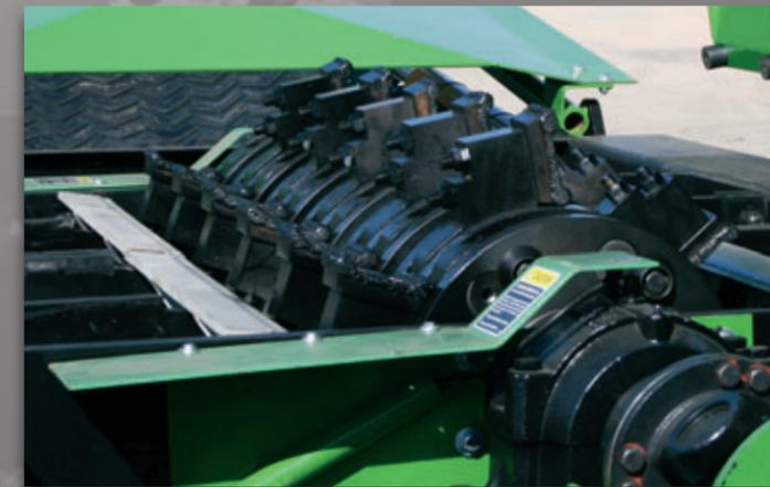
With one of the most aggressive hammermills in the industry, the ProGrind 5200 can cut through mountains of green waste at production rates of over 100 tons-per-hour. ProGrind's special double-bolt hammer tips provide more durability and grinding ease, assuring high production rates, less wear on the hammermill and easy maintenance.
