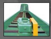
Standard equipment includes TEFC (total enclosed fan cooled) motor, with shaft mounted speed reducer. Allows top performance with lower horsepower than those using sprockets.
